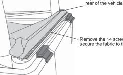
Remove the 14 screws that secure the fabric to the header
